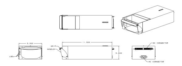
Figure 5-1: Outline Drawing of Power Supply Enclosure
